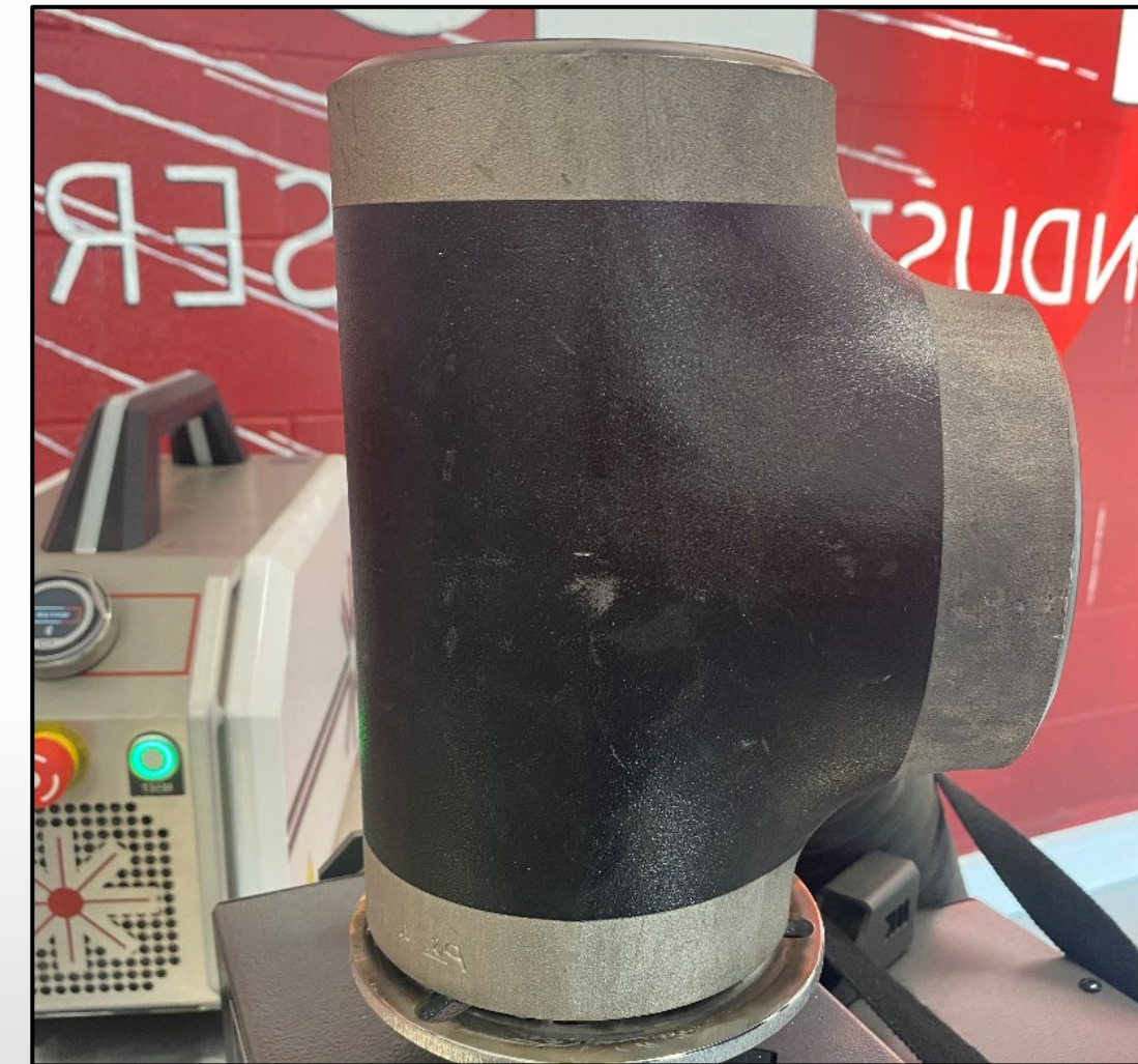
After Laser Cleaning
