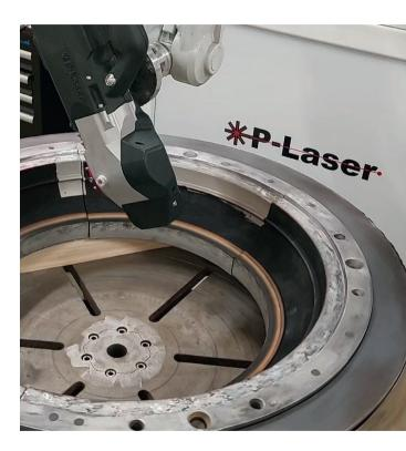
For cleaning tyre moulds, we recommend a QF-500 in an automated setup.
